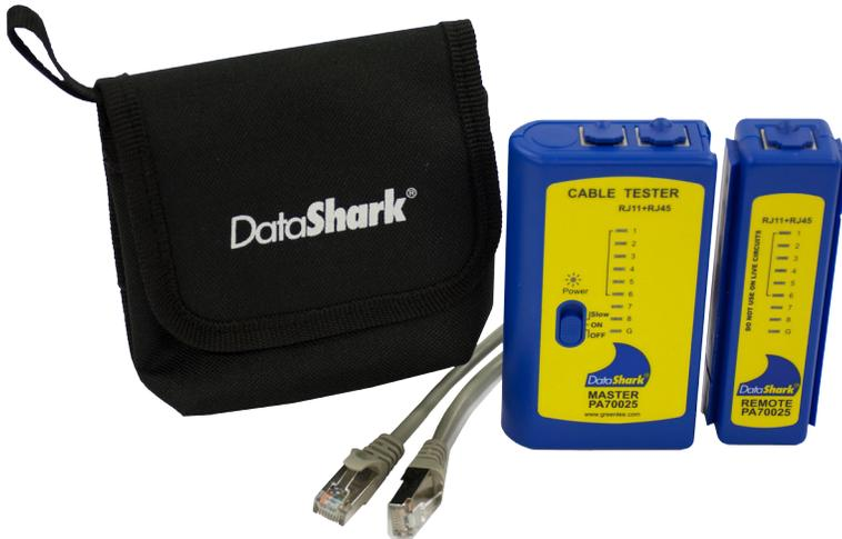
The Data Shark Cable Tester from Greenlee Communications tests the continuity of 8-way (RJ45) data and network and 6-way (RJ11) telephone patch cords and installed cable runs. It maps the cable, line by line and identifies good connections, opens, shorts and crosses. Includes patch cords, 9V battery and carrying pouch.
