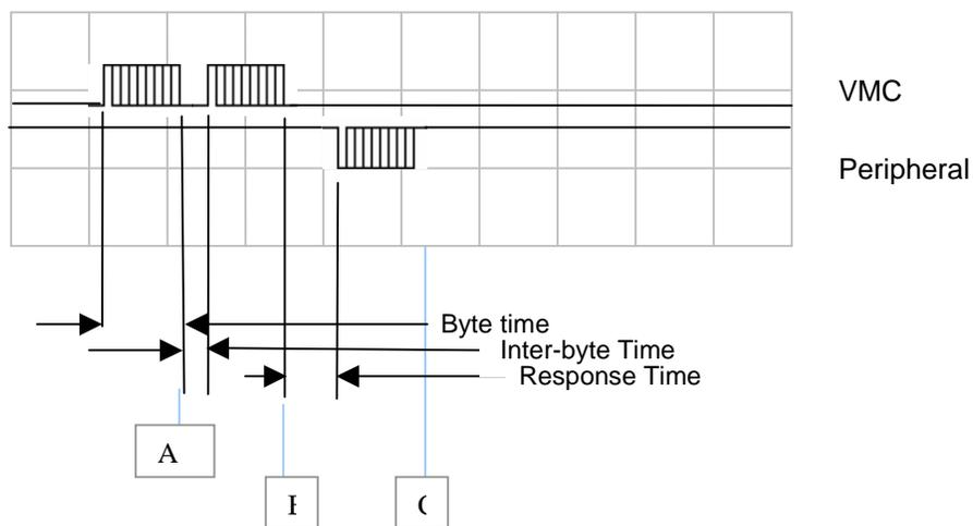
Please note, that the receiving device at the bus (master or slave) will get a receive interrupt (using standard UART devices) only after the byte is fully transmitted. These are the positions A, B, and C in the above diagram.
