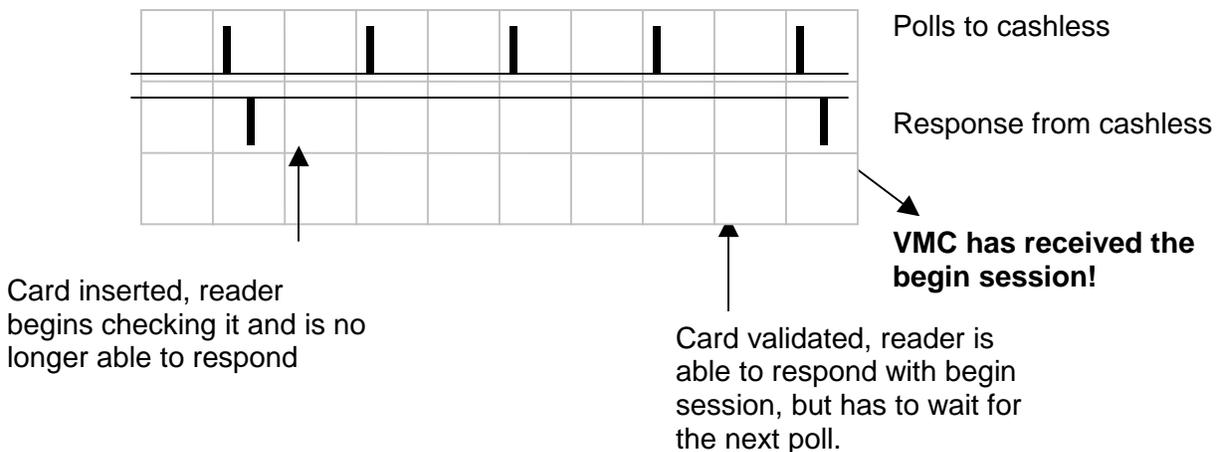
As shown in the above diagram, the time from card insertion to credit being displayed on the vending machine is not specifically related to the polling rate. After the card is inserted, the card reader validates the card. During this time, some card readers are no longer able to answer the poll, others answer with an ACK only.
